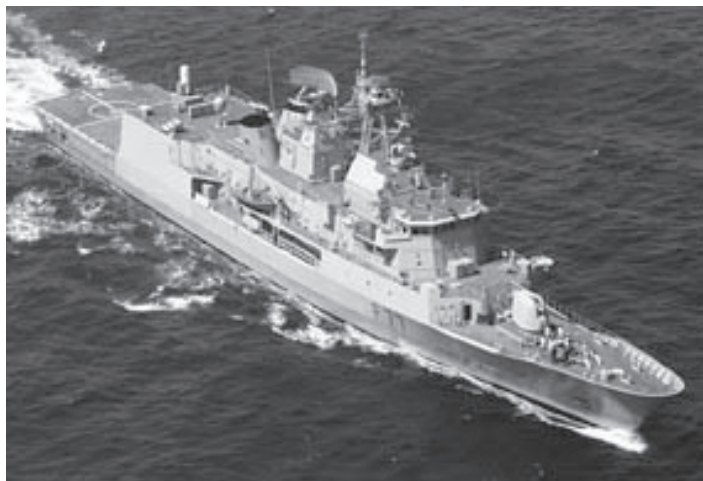
Te Mana 385 ft long, 46 ft wide, 3543 ton. That's Blackpool's old pennant, F77, Te Kaha has F111. A South African Meko class 'Mendi' has F148.
